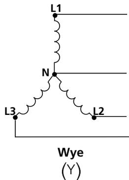
A Delta PDU would use a NEMA L21-30P (the mating Wye plug), but would not use a neutral inside the PDU. This is a perfectly acceptable practice. For example, a data center could deploy Delta PDUs to racks where there is only a need for 208V and Wye PDUs to racks where there is a need for both 120V and 208V.
